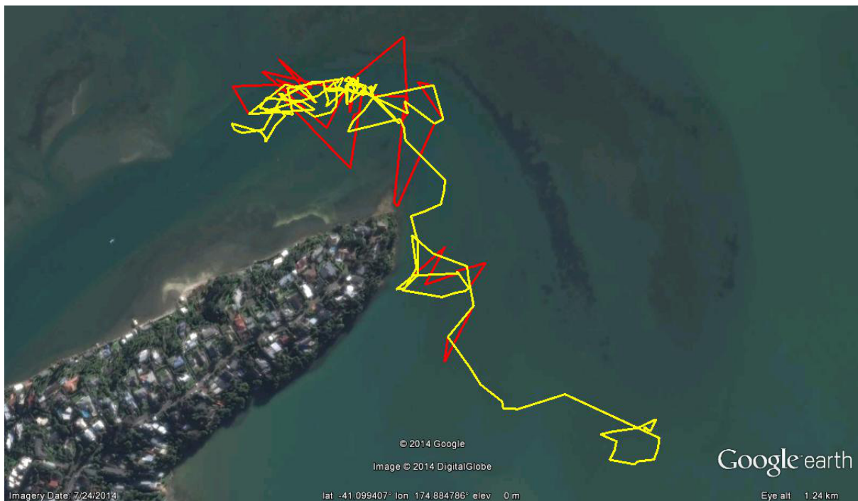
Figure 6: A five hour filtered track of a rig is shown in yellow, the outlying points (shown in red) were removed by using 'altitude' as a filter.
