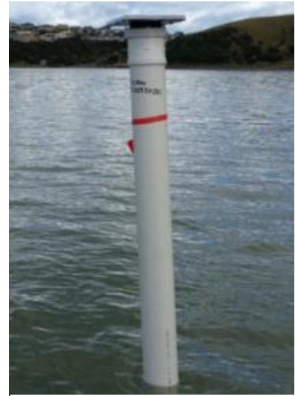
Figure 4: Tall routers with the electronics positioned high above the water.
