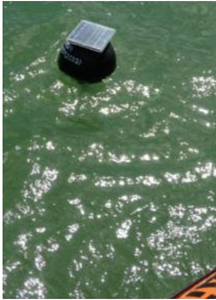
Figure 3: Round router with electronics positioned at or below water level.
